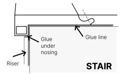
All trims or skirting must be fitted with a 1mm clearance gap above the flooring to allow for the correct raft movement. Trims or skirting must not be fitted to the flooring product. The 1mm gap must not be caulked or siliconed in any way.
