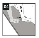
Afterwards press slightly along the short end just installed.
