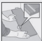
**Fig 1.** First plank, first row. Place a spacer of 15mm thickness to the left and position the plank against the wall. Later, after 3 rows, you can easily position the flooring against the front wall with distances  $\approx$  15mm.
