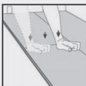
**Fig 8c.** As it flattens itself to the floor, press or gently tap the top of the short end of the installed panel until it clicks. Finish installing this plank by tapping it with a tapping block on the long side to ensure secure installation.
