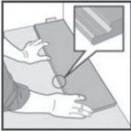
**Fig 1.** First plank, first row. Place a spacer of 15mm thickness to the left and position the plank against the wall. Later, after 3 rows, you can easily position the flooring against the front wall with distances ≈ 15mm.
