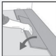
**Fig 7b.** Fold the panel down in a single action movement with a slight press to the left to the short end of the previous panel. Again using the tapping block tap it against the long end into the previous row. During the fold down, make sure the panels are tight against each other
